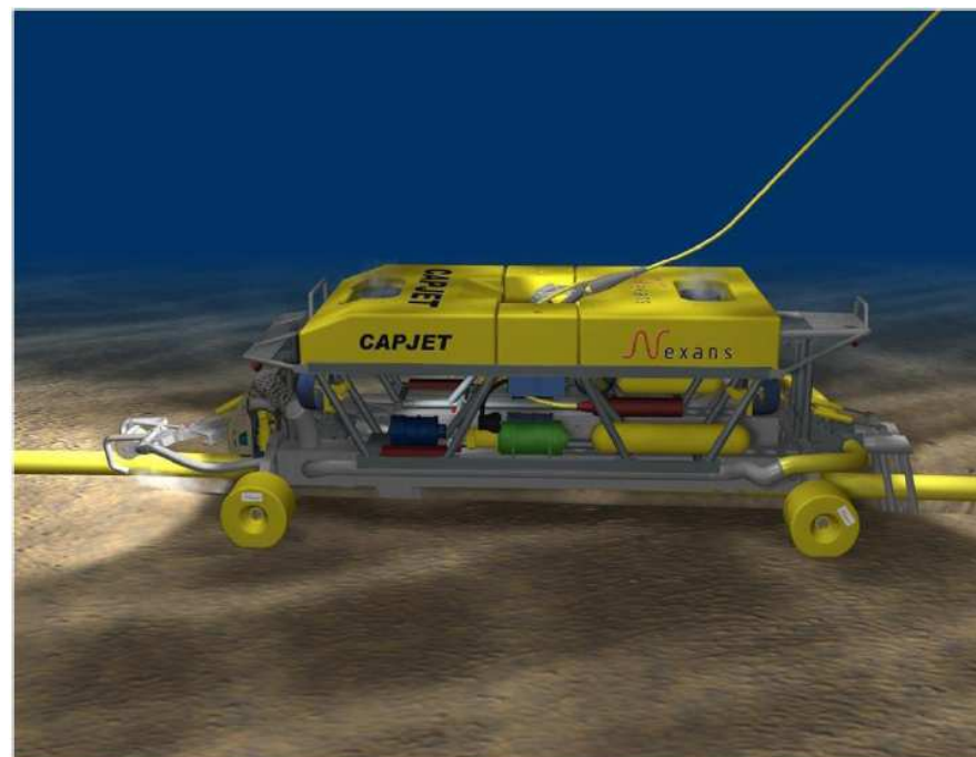
Water jet machine for the silting up of cables
